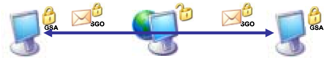
Figure 7: An SGO Encrypted by a GSA Stays Secure Without Any Special Servers or Connections.
