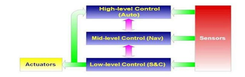
Autopilot Architecture - Source: Unmanned Dynamics, LLC - <u>http://www.u-dynamics.com/sensor\_fusion/sensor.htm</u>
