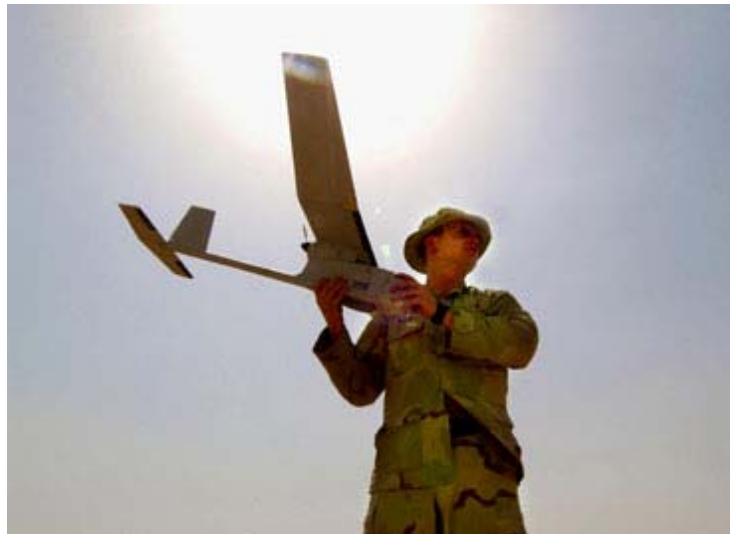
Figure 7 - The proliferation of small UASs, such as this Army Raven, presents a considerable challenge to airspace managers (US Army Photo)
