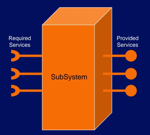
A service is defined by Data format Protocol/carrier, eg DDS Rate and volume Number of allowed connections Access protocols etc
