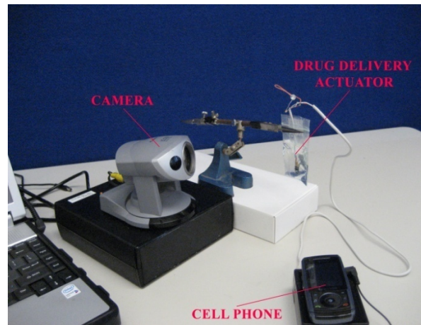
Figure 3. Network-controlled drug actuator setup
