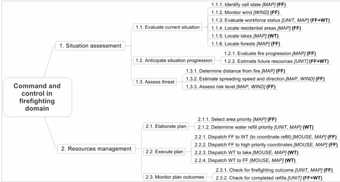
Figure 3. HTA representation, with tasks associated to specific roles and tools. FF = firefighting role, WT = water-provisioning role, MAP = Geospatial information display, UNIT = Unit information panel, WIND = Wind information panel, MOUSE = Computer mouse.
