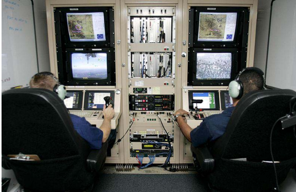
Figure 1. The human factor in UAV operation via ground control station (GCS) displays (reproduced from U.S. Customs and Border Protection (CBP)).
