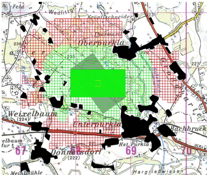
Figure 11: Determination of visibility zones and fire zones based on a given position area. Green cells indicate visible areas which can also be reached by direct fire (i.e. with the given type of weapon system). Red cells indicate areas which are still visible but cannot be reached by fire. Given the center of the position area (green rectangle) other alignments (grey rectangle) are possible. The consideration of different possible alignments may extend the calculated zones.
