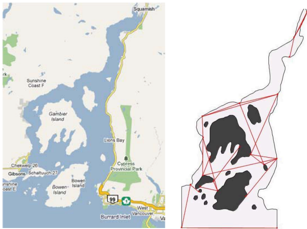
(a) Map of Howe Sound. (b) 22 patrols (guards) with unlimited range sensors cover Howe Sound. Lines show visibility between guards.
