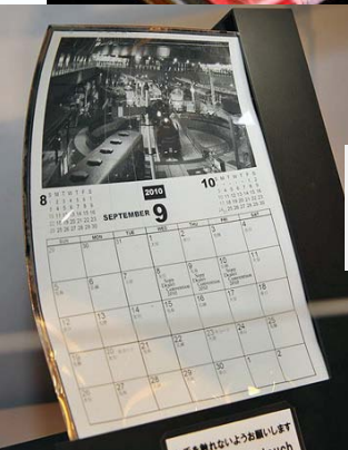
Sony's Rollable OLED display
