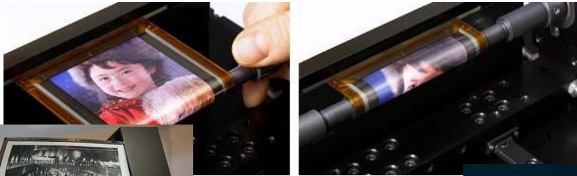
Sony's Rollable OLED display
