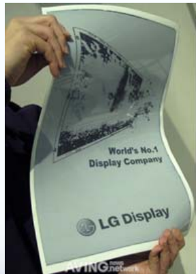
LG'S 19-in flexible display
