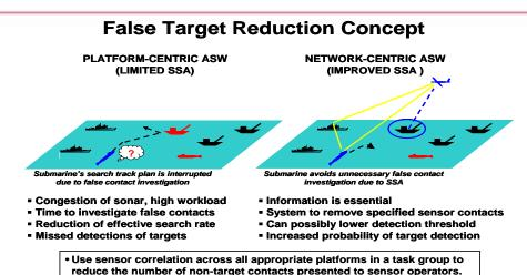
Reduce non-object false contacts, such as reverberation spikes and wrecks, by using acoustic models, in situ data, and local data bases.
