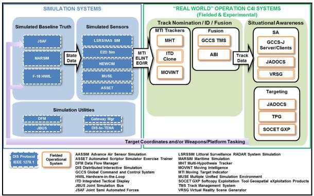
Figure 1.2. Simulation-C4I Architecture
