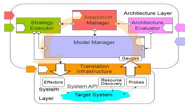
**Image 1:** The Rainbow Framework (from [18]) consists of four primary components: The Model Manager, the Architecture Evaluator, the Adaptation Manager, and the Strategy Executor. In addition, for each target system being managed, there is a Translation Infrastructure that provides the means to send data to the Rainbow framework and for Rainbow to effect changes in the target system.
