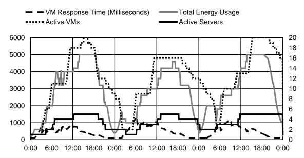
**Figure 6:** The performance of the Rainbow framework with sixty minute intervals between communications. The most degraded communications causes Rainbow to request resources much later than required and keep them activate longer than necessary. The overlapping interaction causes Rainbow to have too many resources online for periods of low activity.
