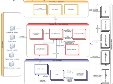
Figure 4 Interoperating Data Sources: Data Flow
