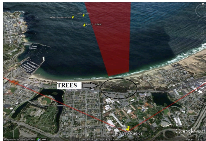
Figure 16. Area affected by high trees between boat and NPS
